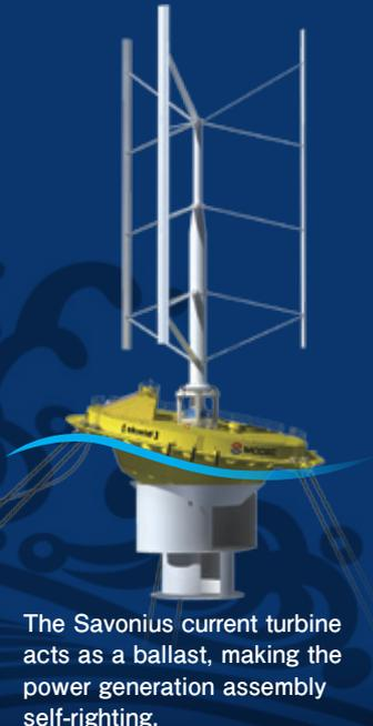
The Savonius current turbine acts as a ballast, making the power generation assembly self-righting.
